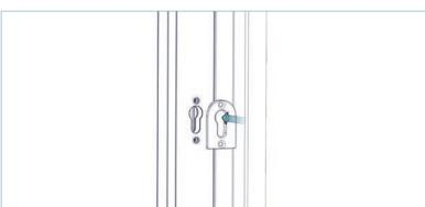
Place the black plastic packer over the cylinder prep and ensure the screw holes line up.
