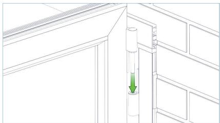
Once the jambs are securely fixed into place, carefully unwrap the sash and lift onto the jamb using the hinge pins to locate it.
