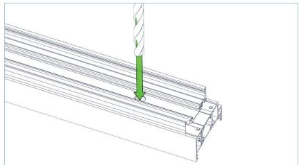
3. From the bottom of the jamb, measure and then drill fixing holes through the first layer of polyamide using a 13mm drill bit. Make sure the hole aligns with the centre of each jamb packer.
