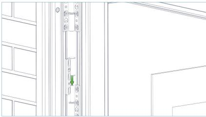
Find the separately provided hinge leaf and slide onto the exposed hinge pin.
