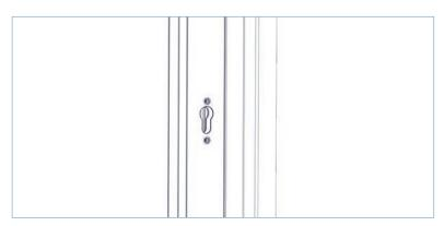
Find the cylinder prep with the riv-nuts in the sash on the locking side. (If retrofitting, you will need to remove the cylinder escutcheon and retaining packer behind it by removing the screws).
