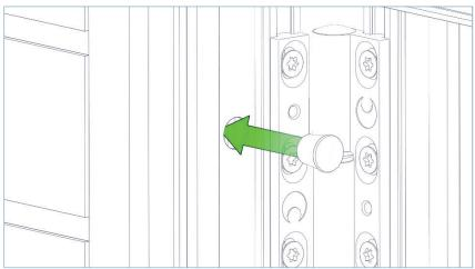
20. Insert the fixing plugs to cover up the fixing holes in the jambs.
