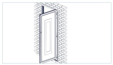
15. Check all the hinge pins are correctly engaged in the hinges.
