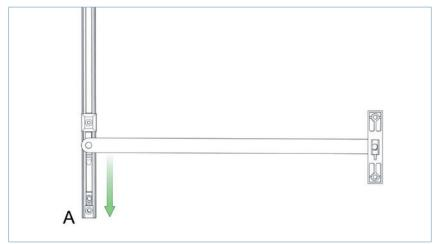
Ensure the slider stop is engaged by placing point (A) against a hard surface and pushing down on the restrictor arm. This will require some force and should result in a click. The restrictor arm should no longer be able to slide up and down the slider housing once this step has been completed.
