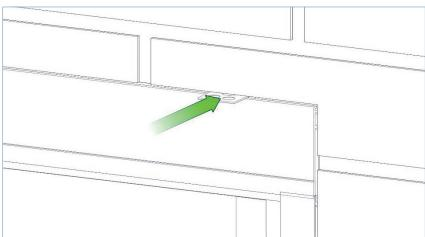
When level, pack out the top of the frame using the appropriate packers. Ensure this is tight but not over compressing the jamb to track connectors.
