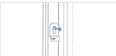
Insert the cylinder and secure using screw through the multi-point lock faceplate.
