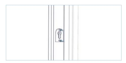
Using the screws provided, ensure the plastic packer is firmly screwed into the riv-nuts.
