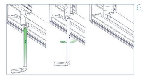
Insert four of the restrictor blocks positioned at the points you have marked on the top track. Do this by using an 8mm Allen key to insert the block into the track and twisting 90° clockwise to lock it in to place. The 5th restrictor block is then inserted half way between the other blocks.
