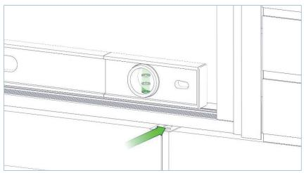
First, using frame packers, ensure the threshold is perfectly level.
