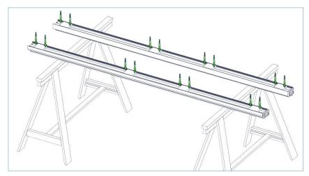
Secure the jamb packers using a 25mm self-tapping screw either side. Ensure each of the jamb packers are positioned and secured correctly. Position fixings within 150mm of the corner. Centre fixings should be spaced 600mm apart thereafter.
