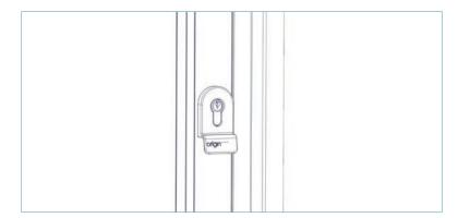
7. The cylinder pull is now fully installed.
