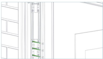
Carefully secure the hinge leaf to the jamb using the provided screws.
