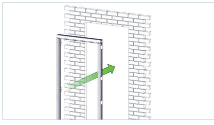
Position the outer frame into the opening, being careful not to scratch any of the profile
