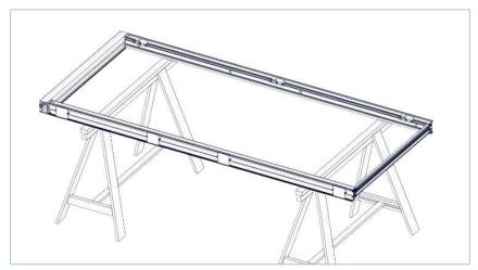
The outer frame should now be assembled and secured together.
