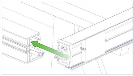
Starting with the top, slide the two jambs into the top track.
