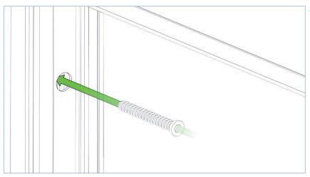
Using the door as a gauge, ensure the locking jamb runs parallel to the edge of the door with the correct spacing (approximately 4mm). Once this is achieved, pack out the jamb and secure using appropriate fixings.
