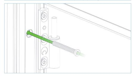
Starting with the hinge side, pack out the jamb so it is perfectly level and secure through the fixing holes prepared earlier using appropriate fixings.
