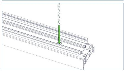
Then, through the 13mm hole, drill an 8mm hole through the remaining jamb and jamb packer.
