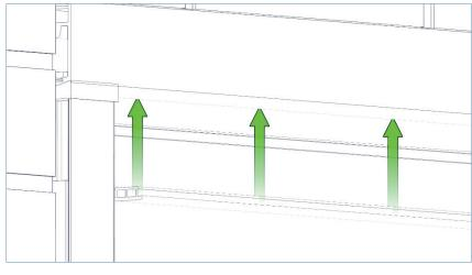
Insert the track gap gasket into the bottom edge of the track.
