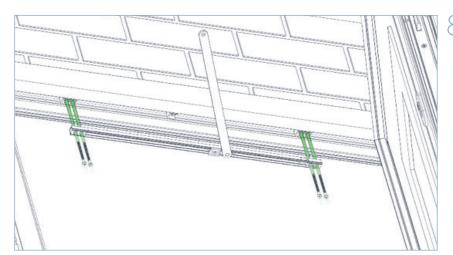
Now place the slider casing back into the top track at your marked position, and secure the last 4 restrictor blocks through the slider casing using the 5.0 x 60mm screws as shown. It may help to disconnect the sash pivot at this point for ease of installation. Once the screws have been fitted reconnect the sash pivot. Check the door for proper operation.
