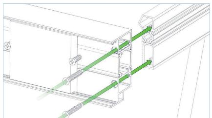
For the mobility threshold, secure the jambs to the threshold using two of the supplied 3.5mm screws. Seal the mating faces with silicone. If it is a standard threshold, repeat step 7.
