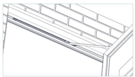
5. Insert the slider casing into the top track making sure it is still connected to the sash pivot, it should only fit in one position. Then, using a non-permanent method, mark the positions of the four screw holes in the slider casing, then move the slider casing out of the way.
