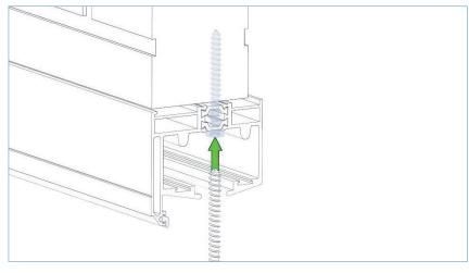
Using appropriate fixings, secure the top track through the polyamides.
