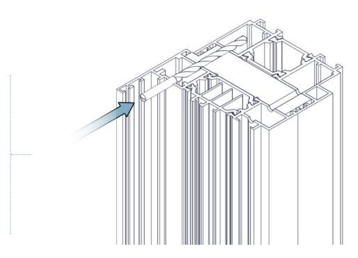
Using supplied screws, fix the window frame to the door jamb through the jamb packers
